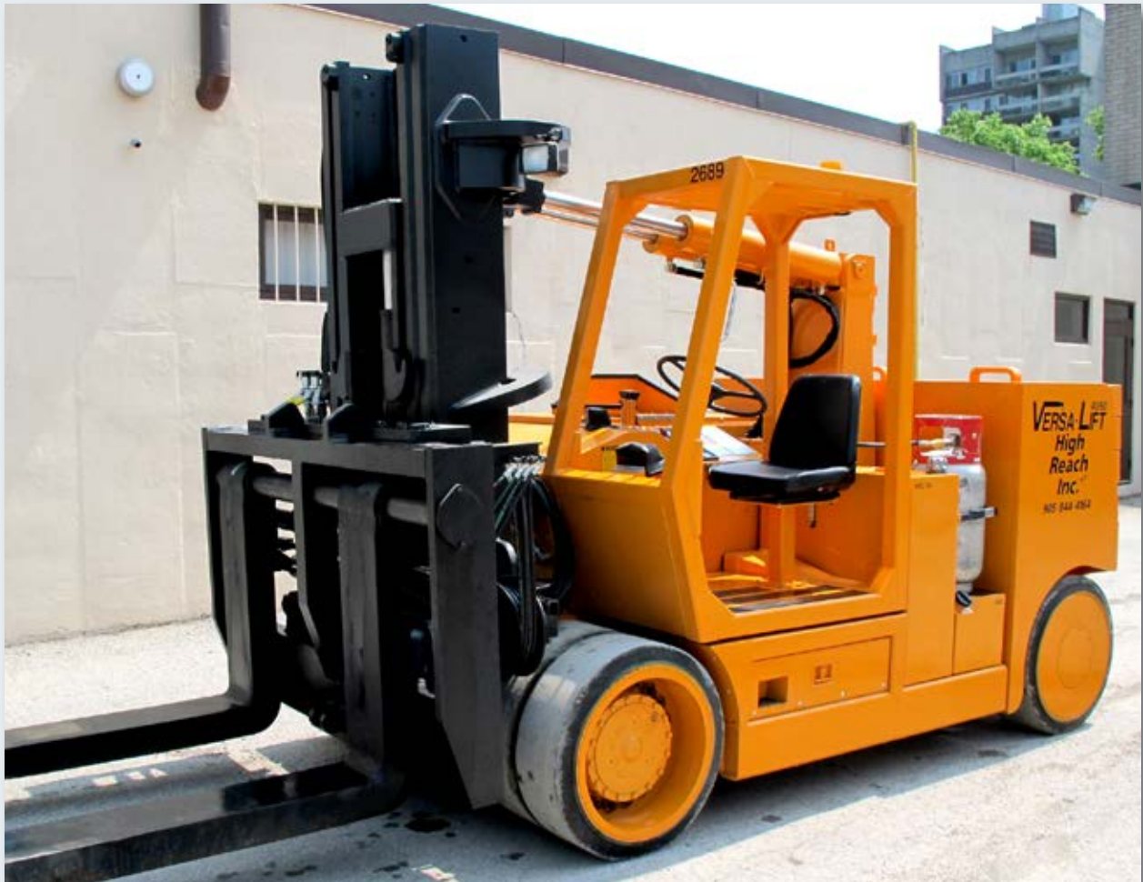
Versa-Lift 40-60: 60,000 lbs capacity.
